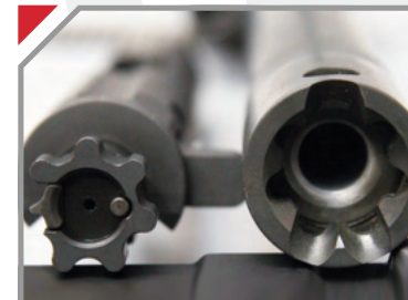
CHAMBER: Sustained-Fire bolt and barrel extension feature tangential radii at lug roots and tips to reduce stress and increase shear strength for heavy-duty performance.
