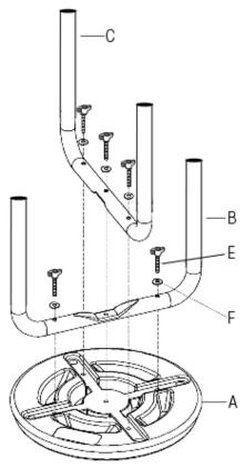
Tighten all five (5) Wingnut Screws (E) until secure in the seat.
