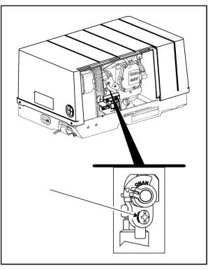
FIGURE 12. CARBURETOR FLOAT BOWL DRAIN VALVE
