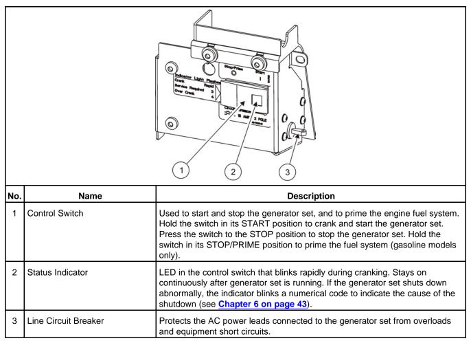
FIGURE 3. GENERATOR SET CONTROL PANEL
