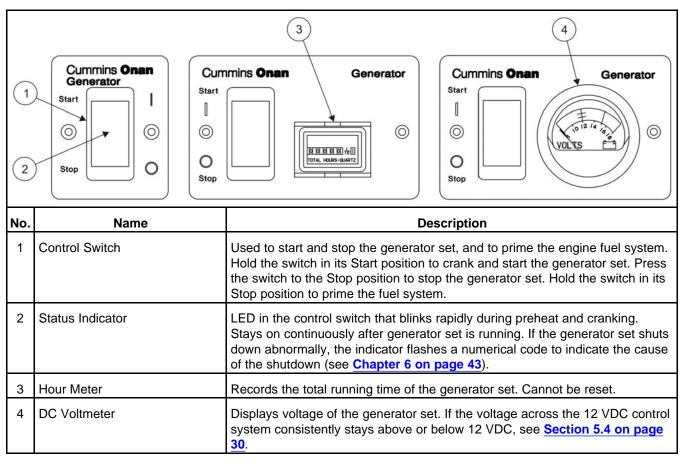
FIGURE 4. REMOTE CONTROL PANELS
